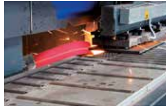
Mechanical bevel cutting
