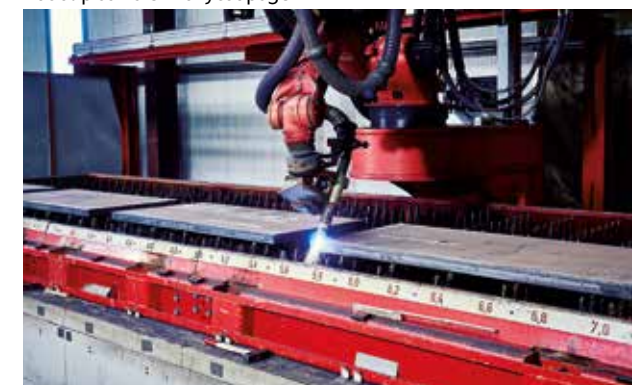
Robot plasma 3D/oxycoupage
