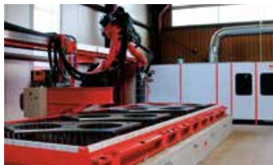
Robot plasma 3D/oxycoupage
