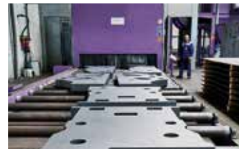
Continuous blasting machine
